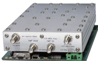
SC5303A – 1 MHz to 1.3 GHz RF Downconverter
