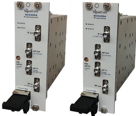
SC5305A & SC5405A – 1 MHz to 3.9 GHz RF Downconverter and Upconverter
